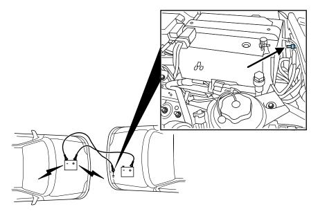
4. Make the final connection of the negative (-) cable to the ground stud located toward the front of the vehicle (forward of the battery) on the radiator support. Keep the negative (-) cable away from the battery and the carburetor/fuel injection system.
